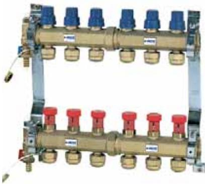
Top Control manifolds Ø 1¼" are made of brass and used to distribute piping. They are equipped with shut-off valves (suitable for electrothermal heads), micrometric lock-shield valves with data plates to locate rooms, ball air valves and ball wash-out valves with rubber-holders and plugs, brackets with vibration-damping rubber tops, which can be installed into cabinets or fixed to the wall, and fittings for 14-10, 17-13 or 20-16 polyethylene pipes.
